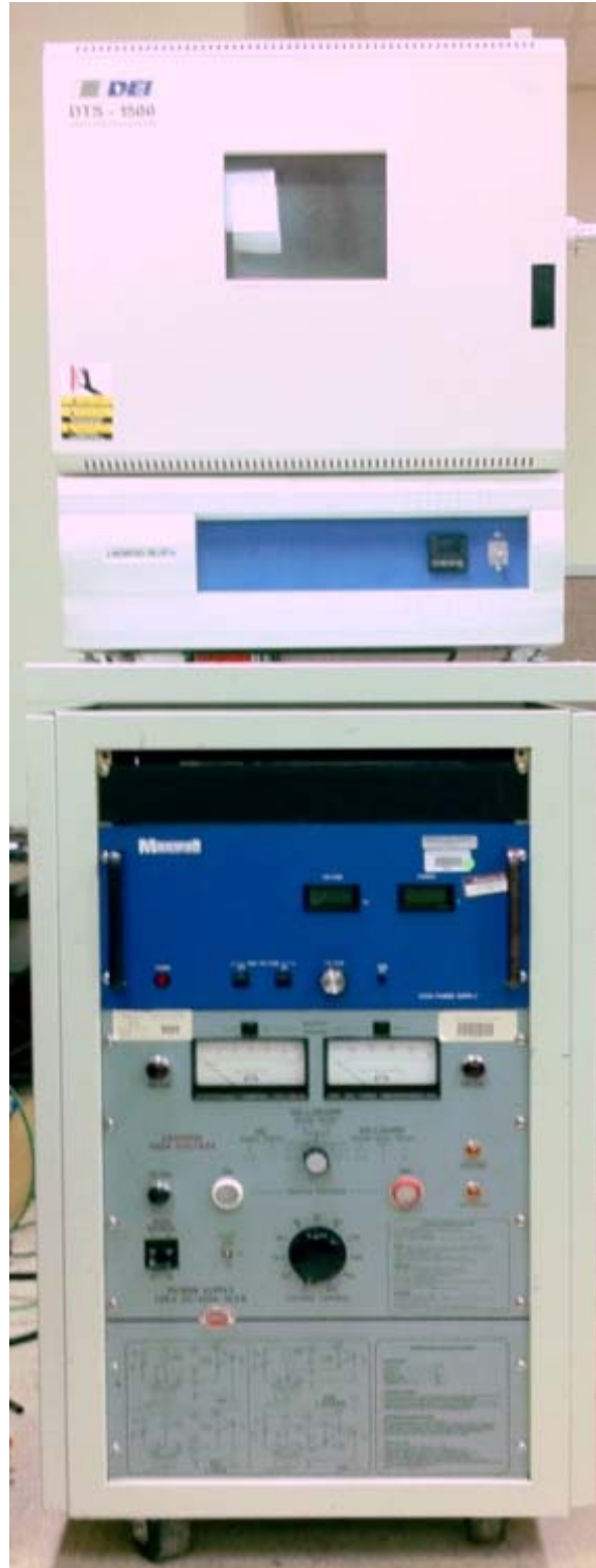
Figure 6.1 The Dielectric Test System
